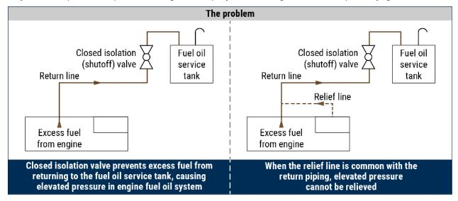
Simplified diagram of a diesel engine fuel system, showing a return line with closed isolation (shutoff) valve and relief line common with return piping system.
